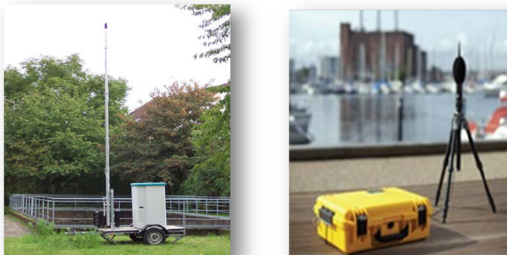
Figure 18: Noise Monitoring Terminals (NMTs) – on trailer (left), portable (right)
